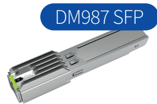
XGS-PON ONU in SFP+ form factor
