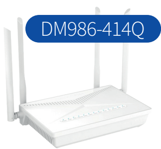
ONU GPON with 4 GE LAN ports, 1 voice port, and Wi-Fi AC1200
